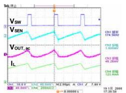
Fig 47. Switching waveform  $(12V_{IN}, 3.6V_{OUT}, R_{SEN}=0.27)$
