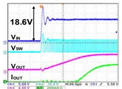
Fig 52. C<sub>IN</sub>=C<sub>OUT</sub>=Ceramic capacitor (2 x 4.7uF/35V)
