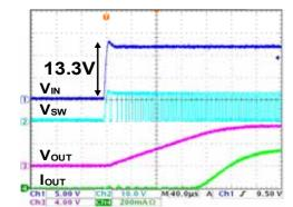
Fig 51. C<sub>IN</sub>=C<sub>OUT</sub>=Tantalum capacitor (10uF/50V)
