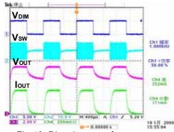
Fig 46. Dimming waveform (V<sub>IN</sub>=12V, R<sub>SEN</sub>=0.27 , 2-LED)
