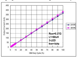
Figure 59. DIM duty cycle: 1% ~ 100%
