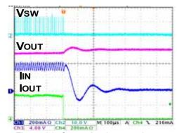
Figure 61. Open-circuit protection
