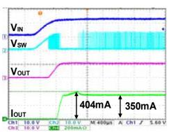
Figure 58. The start-up waveform @  $V_{IN}$ =12V,  $V_{OUT}$ = 10.8,  $R_{SEN}$ =0.27
