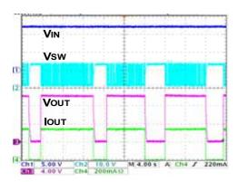
Figure 63. Thermal protection
