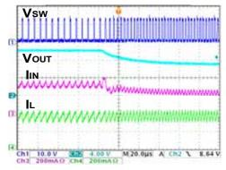
Figure 62. Short-circuit protection
