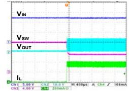
Fig 53. C<sub>IN</sub>=C<sub>OUT</sub>=Tantalum capacitor (10uF/50V)
