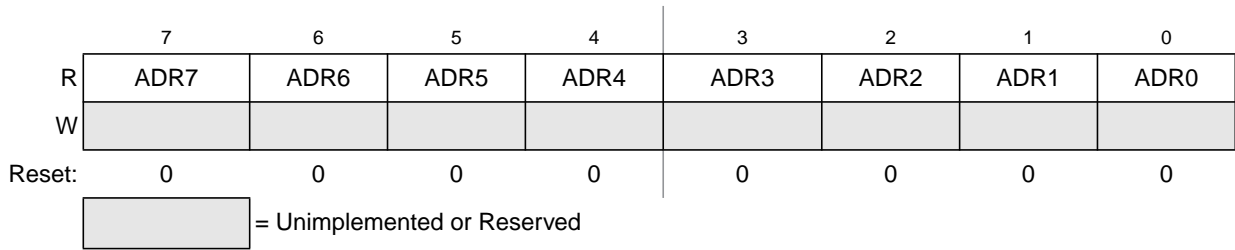
Figure 9-7. Data Result Low Register (ADCRL)
