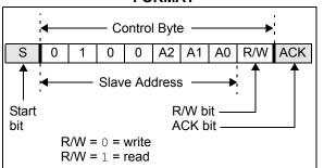
FIGURE 1-3: SPI CONTROL BYTE
