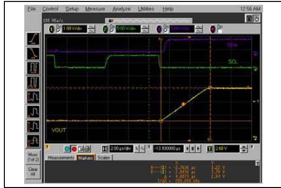
FIGURE 2-98: Half-Scale Settling Time (400h to C00h) (MCP4726).
