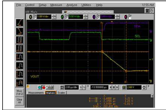
FIGURE 2-99: Half-Scale Settling Time (C00h to 400h) (MCP4726).
