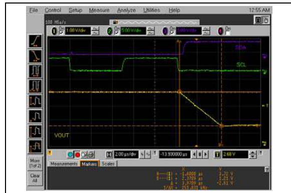
FIGURE 2-99: Half-Scale Settling Time (C00h to 400h) (MCP4726).
