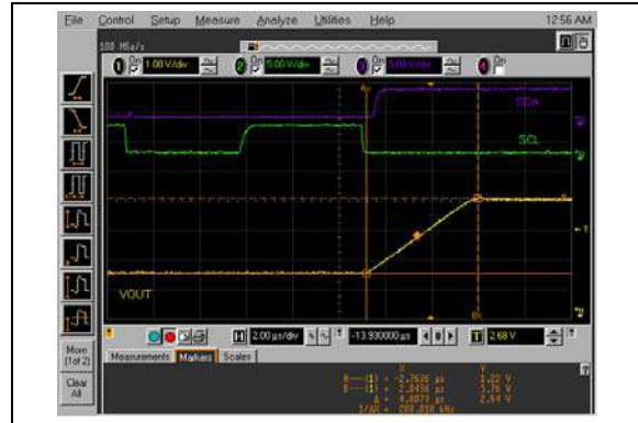
FIGURE 2-98: Half-Scale Settling Time (400h to C00h) (MCP4726).
