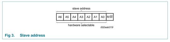
The last bit of the address byte defines the operation to be performed. When set to logic 1 a read is selected, while a logic 0 selects a write operation.
