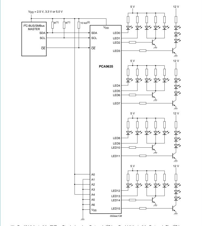
(1)  $R = 10 k\Omega$  (typical) for SMBus, Standard-mode or Fast-mode I<sup>2</sup>C-bus.  $R = 1 k\Omega$  (typical) for Fast-mode Plus I<sup>2</sup>C-bus.
