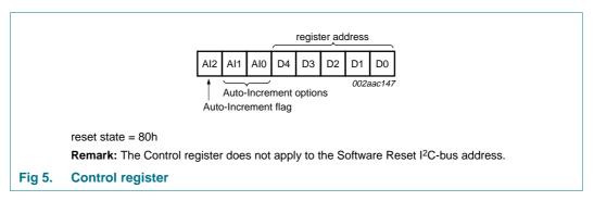
When the Auto-Increment flag is set (Al2 = logic 1), the five low order bits of the Control register are automatically incremented after a read or write. This allows the user to program the registers sequentially. Four different types of Auto-Increment are possible, depending on Al1 and Al0 values.
