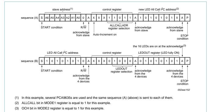
Fig 15. LED All Call I<sup>2</sup>C-bus address programming and LED All Call sequence example
