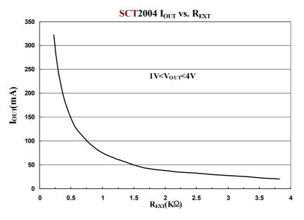
According to SCT2004' I-V curve, the output voltage should be larger than 1V to get 320 mA constant current. By applying proper output voltage, the SCT2004' output current set by an external resistor is approximate to:  $I_{OUT} = 120(630 / \text{REXT})$  (mA) (chip skew < ±6%). Thus the output current is set to be about 84mA at REXT = 900 $\Omega$ .
