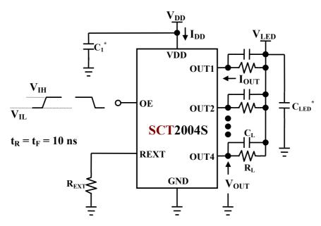
\* Place the  $C_1/C_{LED}$  more close to IC VDD/OUT pin(not power supply) as possible.
