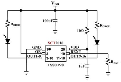
(2) Lighting with  $V_{LED} > 5V$ , e.g.  $V_{LED}=12V/24V$
