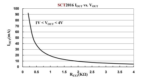
Furthermore, when SCT2016's output voltage is set between 1 Volt and 4 Volt, the output current can be estimated approximately by:  $I_{OUT} = 30(630 \ / \ R_{EXT})$  (mA) (chip skew < ±6%). Thus the output current are to be set about 21mA at  $R_{EXT} = 900\Omega$ .
