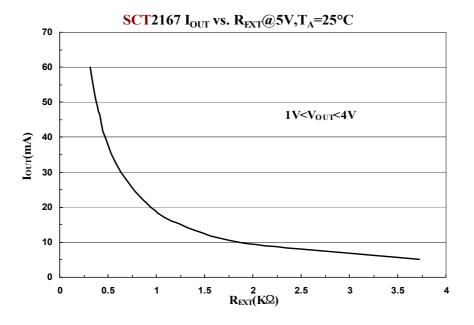
According to SCT2167' I-V curve, the output voltage should be larger than 1V to get 45 mA constant current. By applying proper output voltage, the SCT2167' output current set by an external resistor is approximate to:  $I_{OUT} = 30(630 / \text{REXT})$  (mA) (chip skew < ±5%). Thus the output current is set to be about 21mA at REXT = 900 $\Omega$ .
