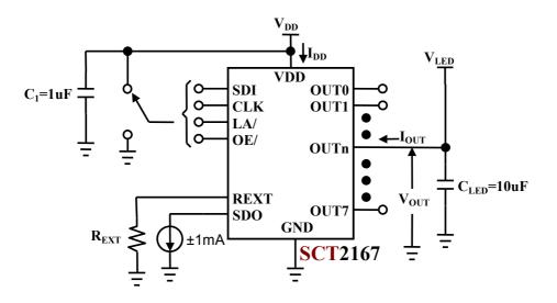
\*Place C<sub>1</sub>/C<sub>LED</sub> as close to IC VDD/OUT pin(not supply source) as possible.
