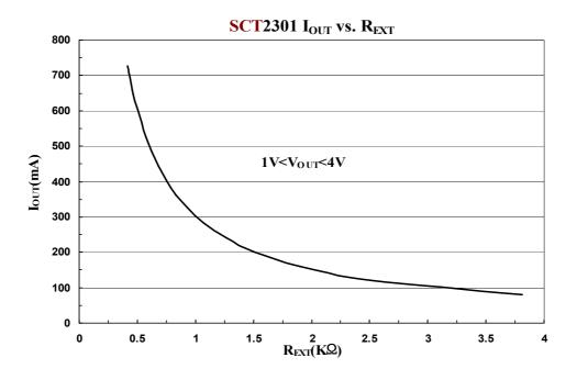
Furthermore, when SCT2301's output voltage is set between 1 Volt and 4 Volt, the output current can be estimated approximately by:  $I_{OUT}$  = 480(630 /  $R_{EXT}$ ) (mA) (chip skew < ±4%). Thus the output current are set about 336mA at  $R_{EXT}$  = 900 $\Omega$ .
