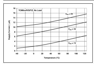
**FIGURE 2-1:** Supply Current vs. Temperature.
