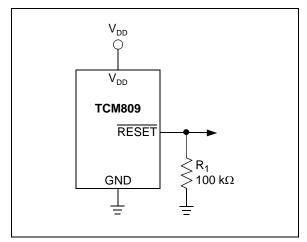
**FIGURE 4-2:** The addition of  $R_1$  at the <u>RESET</u> output of the TCM809 ensures that the <u>RESET</u> output is valid to  $V_{DD} = 0V$ .
