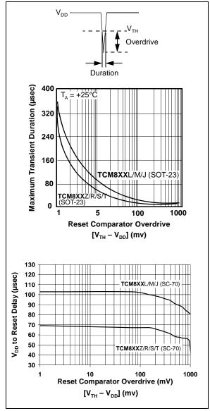
FIGURE 4-1: Maximum Transient Duration vs. Overdrive for Glitch Rejection at +25°C.
