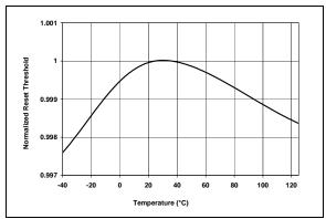
**FIGURE 2-4:** Normalized Reset Threshold vs. Temperature.
