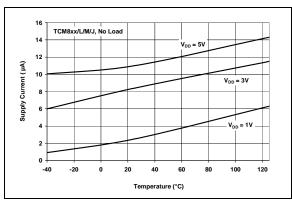
**FIGURE 2-2:** Supply Current vs. Temperature.
