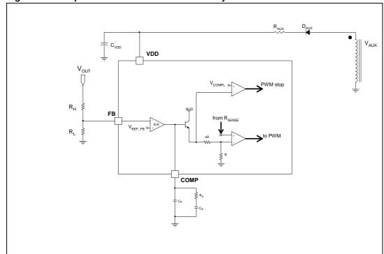
Figure 27. FB pin connection for non-isolated fly-back
