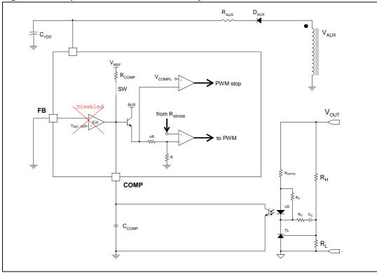
Figure 28. FB pin connection for isolated fly-back
