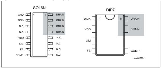
Note: The copper area for heat dissipation has to be designed under the DRAIN pins.
