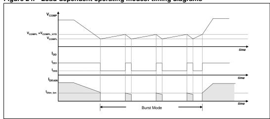
Figure 24. Load-dependent operating modes: timing diagrams
