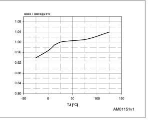
Figure 12. Operating supply current (switching) vs T<sub>.1</sub>
