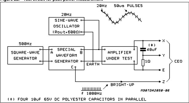
Figure 22. Test circuit for peak power measurement
