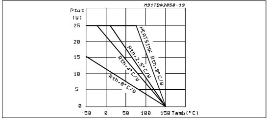
Figure 20. Maximum allowable power dissipation vs. ambient temperature
