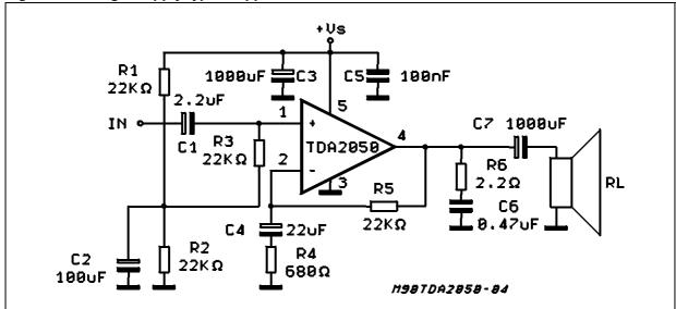
Figure 6. Single-supply typical application circuit
