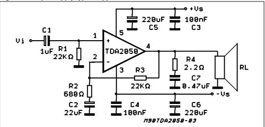
Figure 4. Split-supply typical application circuit
