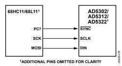
Figure 35. AD5302/AD5312/AD5322 to 68HC11/68L11 Interface
