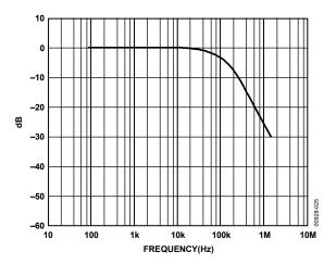
Figure 25. Multiplying Bandwidth (Small-Signal Frequency Response)
