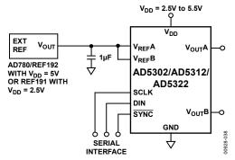
Figure 38. AD5302/AD5312/AD5322 Using External Reference
