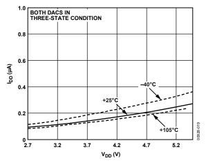
Figure 19. Power-Down Current vs. Supply Voltage
