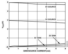
Figure 16. Source and Sink Current Capability
