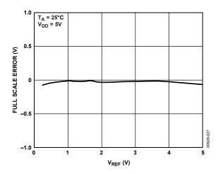
Figure 27. Full-Scale Error vs. V<sub>REF</sub> (Buffered)
