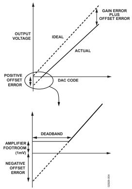
Figure 3. Transfer Function with Negative Offset
