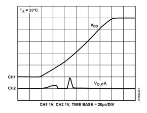
Figure 22. Power-On Reset to 0 V
