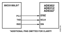
Figure 36. AD5302/AD5312/AD5322 to 80C51/80L51 Interface
