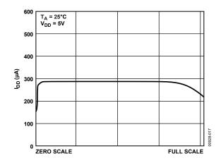
Figure 17. Supply Current vs. Code
