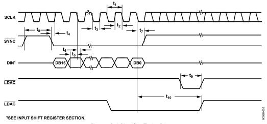
Figure 2. Serial Interface Timing Diagram
