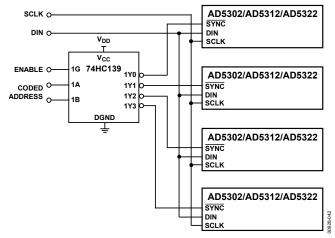
Figure 42. Decoding Multiple AD5302/AD5312/AD5322 Devices in a System
