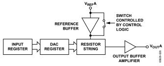
Figure 28. Single DAC Channel Architecture
