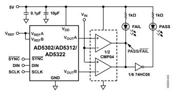
Figure 43. Window Detector Using AD5302/AD5312/AD5322
