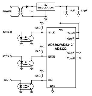
Figure 41. AD5302/AD5312/AD5322 in an Opto-Isolated Interface
