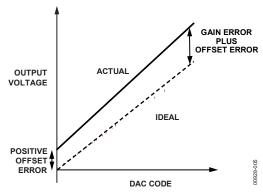
Figure 4. Transfer Function with Positive Offset
