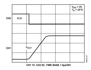
Figure 21. Half-Scale Setting (¼ to ¾ Scale Code Change)
