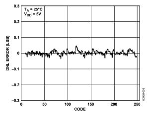
Figure 9. AD5302 Typical DNL Plot
