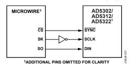
Figure 37. AD5302/AD5312/AD5322 to MICROWIRE Interface
