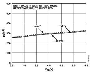
Figure 18. Supply Current vs. Supply Voltage
