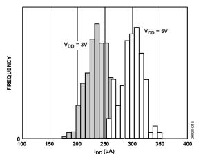
Figure 15.  $I_{DD}$  Histogram with  $V_{DD} = 3 V$  and  $V_{DD} = 5 V$
