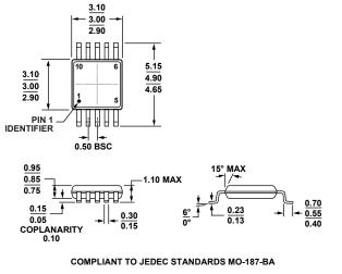
Figure 45. 10-Lead Mini Small Outline Package [MSOP] (RM-10) Dimensions shown in millimeters
