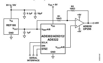
Figure 40. Bipolar Operation Using the AD5302/AD5312/AD5322
