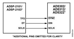
Figure 34. AD5302/AD5312/AD5322 to ADSP-2101/ADSP-2103 Interface
