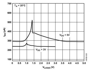
Figure 20. Supply vs. Logic Input Voltage
