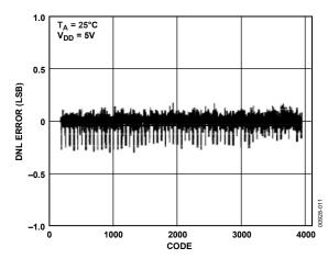
Figure 11. AD5322 Typical DNL Plot
