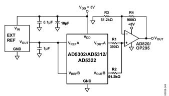
Figure 44. Coarse/Fine Adjustment
