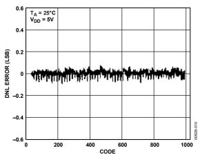
Figure 10. AD5312 Typical DNL Plot
