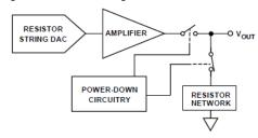
Figure 26. Output Stage During Power-Down
