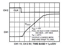
Figure 18. Full-Scale Settling Time
