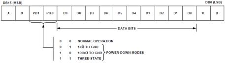
Figure 25. Input Register Contents
