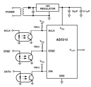
Figure 34. AD5310 with an Opto-Isolated Interface
