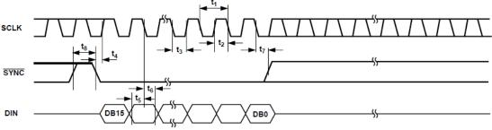
Figure 2. Serial Write Operation
