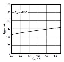
Figure 15. Supply Current vs. Supply Voltage
