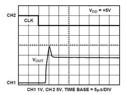
Figure 21. Exiting Power-Down (200 Hex Loaded)
