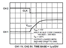
Figure 19. Half-Scale Settling Time
