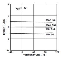
Figure 8. INL Error and DNL Error vs. Temperature
