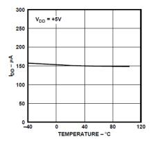
Figure 14. Supply Current vs. Temperature
