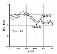
Figure 7. Typical Total Unadjusted Error
