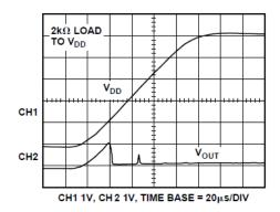
Figure 20. Power-On Reset to 0 V
