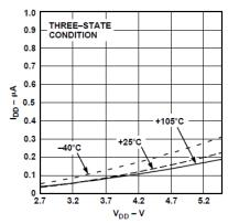
Figure 16. Power-Down Current vs. Supply Voltage
