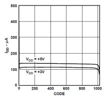
Figure 13. Supply Current vs. Code
