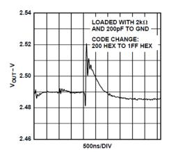
Figure 22. Digital-to-Analog Glitch Impulse
