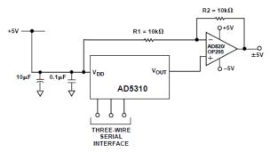
Figure 33. Bipolar Operation with the AD5310
