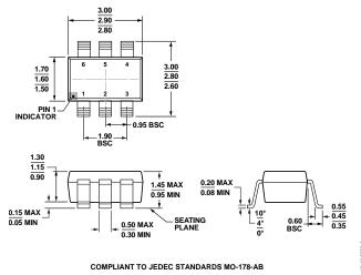
Figure 35. 6-Lead Small Outline Transistor Package [SOT-23] (RJ-6) Dimensions shown in millimeters
