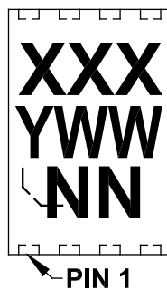
8-Lead TDFN (2x3x0.75 mm)
