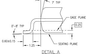
Figure 4. 20-Lead Small Outline Package (SOP), EIAJ TYPE II, 5.3mm Wide
