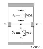
Model of EMI filtering with matched capacitances C<sub>1</sub> and C<sub>2</sub>
