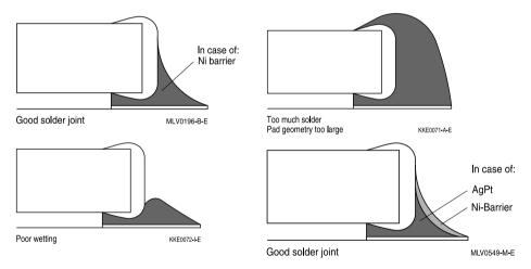
Good and poor solder joints caused by amount of solder in reflow soldering.
