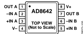
Figure 3. 8-Lead SOIC (R-8)
