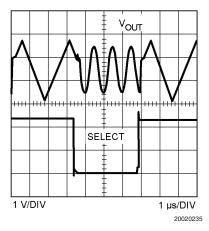
FIGURE 6. 2:1 MUX Output
