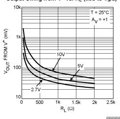
Output Swing from V+ vs. R<sub>L</sub> (tied to V<sub>S</sub>/2)
