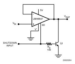
FIGURE 3. Active Pull-Down Schematic
