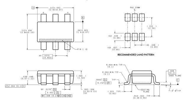
CONTROLLING DIMENSION IS INCH VALUES IN [ ] ARE MILLIMETERS
