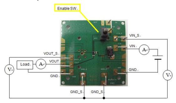
The enable switch has three positions.
